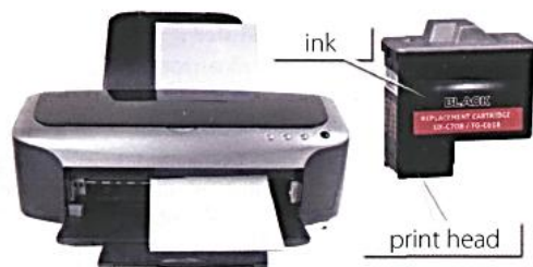
The quality (resolution) of the images goes up to 2,400 dots per inch (dpi)
